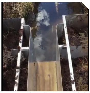
The Living Bog has installed a number of flow measuring structures on selected raised bog project sites. These are used to monitor the discharge and the water quality from the bog. View on YouTube: <a href="https://www.youtube.com/watch?v=p062FiXesFE">www.youtube.com/watch?v=p062FiXesFE</a>
