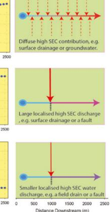
**Figure 3:** Modelled examples of typical water quality profiles along a river reflecting responses to inputs of elevated SEC water under contrasting physical settings (right).
