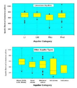
**Figure 1:** Box and Whisker plot of median specific electrical conductances for major Irish bedrock types, analysed as part of the EPA's groundwater monitoring programme. (Above) Limestone aquifers, (Below) Non-carbonate and
