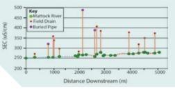
**Figure 4:** Specific Electrical Conductance profile measured along the course of the Mattock River (Co. Louth/Co. Meath), April 2012. The gradual increase in the SEC of river water reflects minor contributions of elevated SEC water discharging from numerous field drains and buried pipes discharging to the Mattock along its course. (Data P.Rafferty, DkIT)
