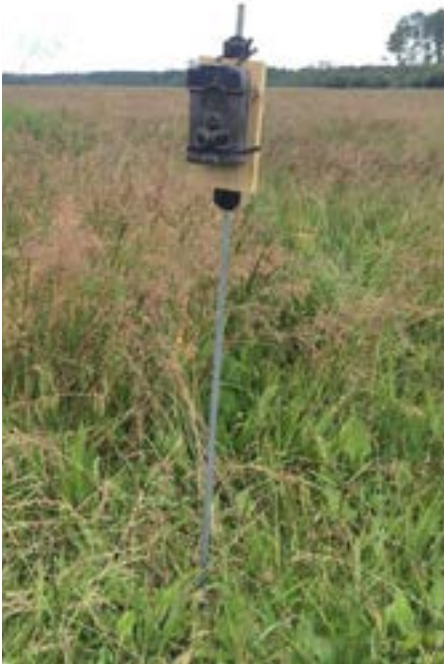
CAMERA TRAP: USED FOR CAPTURING PICTURES OF WILD ANIMALS BASED ON A TRIGGER OR INFRARED SENSOR.
