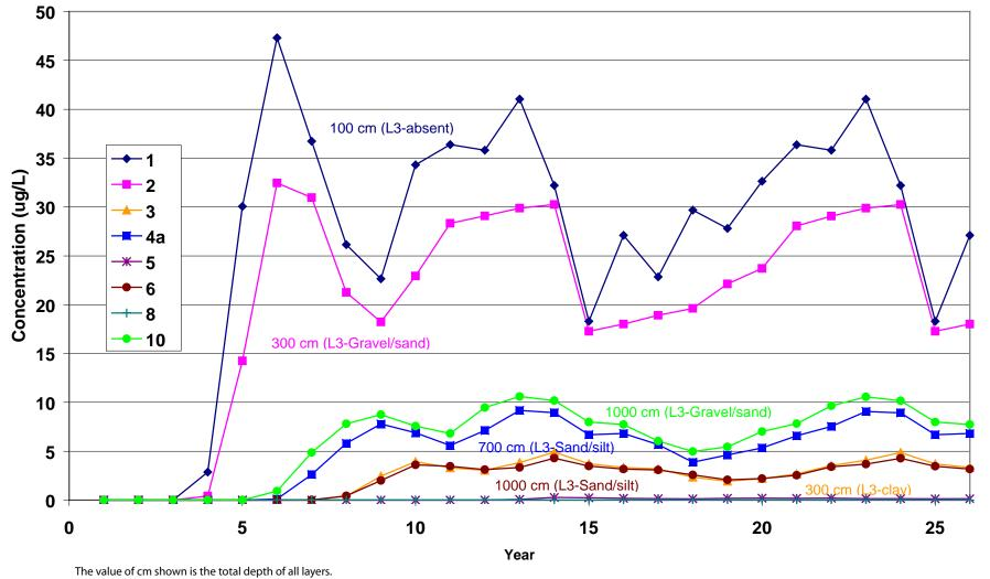
L3" indicates the subsoil type for layer three
