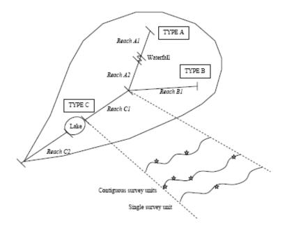
Figure 1: A hypothetical catchment showing the main types of approach to hydromorphological survey, set within the context of river scale ('type', 'reach', 'survey unit') (  $\ddagger$  = survey unit) (CEN Guidance Document TC 230/WG 2/TG 5: N32)
