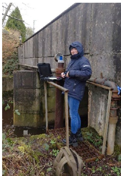
Patricia downloading water level data at Ballyfarnon, Co Roscommon for monitoring compliance with discharge licences in the Feorish Catchment.
