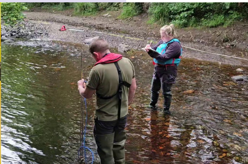
IFI staff monitoring fish and habitat variables (e.g. depth and flow diversity) at a demonstration site where large wood has been re-introduced as habitat restoration measure (River Dodder, Dublin).
